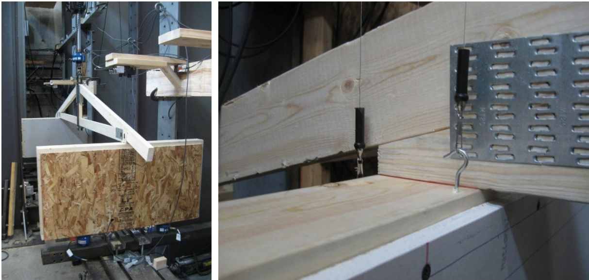
Figure 2. Wall Construction Test Setup
